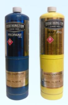
ITE is pleased to offer from stock CYL-P400 and CYL-M-400 gas in non-refillable steel cylinders. Both cylinders are equipped with a CGA 600 valve having 1.000 - 20 UNEF - RH - ext. thread. Constructed of durable steel, the slim, lightweight cylinder is easy to grip and maneuver.
